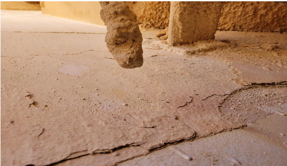
Bottom Flushing System Nozzle - Clogged
