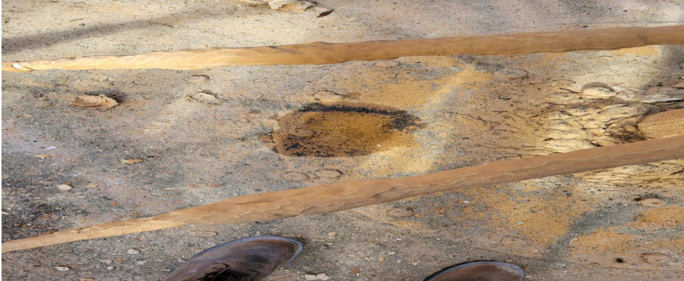
Oil Leak on Impeller & Tie Rods Coated with Calcium Carbonate
