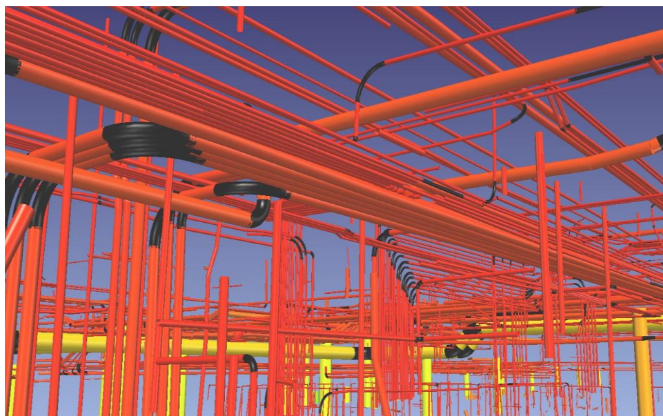
Scan to BIM workflow of existing conditions to building services (MEP/F)
