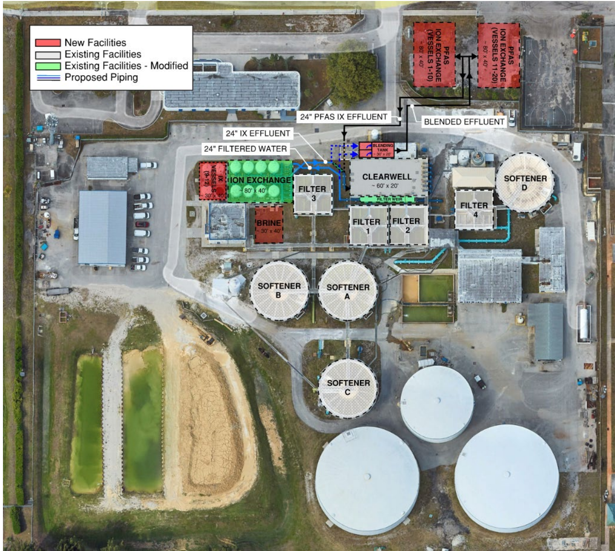
Figure 5.7 Potential Site Layout for Treatment Alternative 2 - Regenerable FIX Process Expansion and the Addition of Pressure Vessels for PFAS Treatment Using IX Resin
