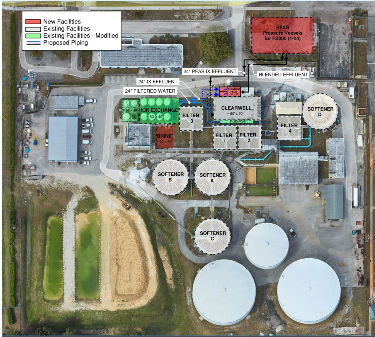
Figure 5.8 Potential Site Layout for Treatment Alternative 3 - Regenerable FIX Process Expansion and the Addition of Pressure Vessels for PFAS Treatment Using FS200
