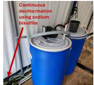
Dechlorination step to preserve the gel-based IX resins
