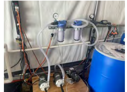
Pretreatment stage (Cartridge filtration) prior to adsorption skid
