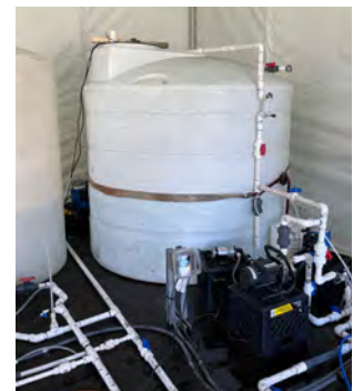
The aeration pilot could be used to test sulfide removal and air stripping of THMs post formation.
