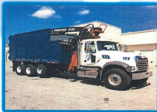
EWS 2017 Mack GU713 with Prentice Boom Loader and 45 yard Collection Body
