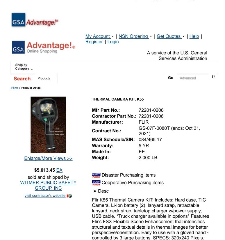
Thermal sensitivity: <30 mL @ 86F. FOV: 51x38 degrees, fixed focus. Image frequency: 60 Hz. 2X digital zoom. FPA/Spectral range: uncooled micro bolometer/7.5-13um. Start-up time: <17 sec (IR-image, no GUI); 4 sec from sleep mode. Stores up to 200 files total of 5 minute
