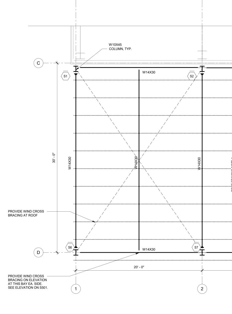
1 ROOF FRAMING PLAN S202 SCALE: 1/4" = 1'-0"
