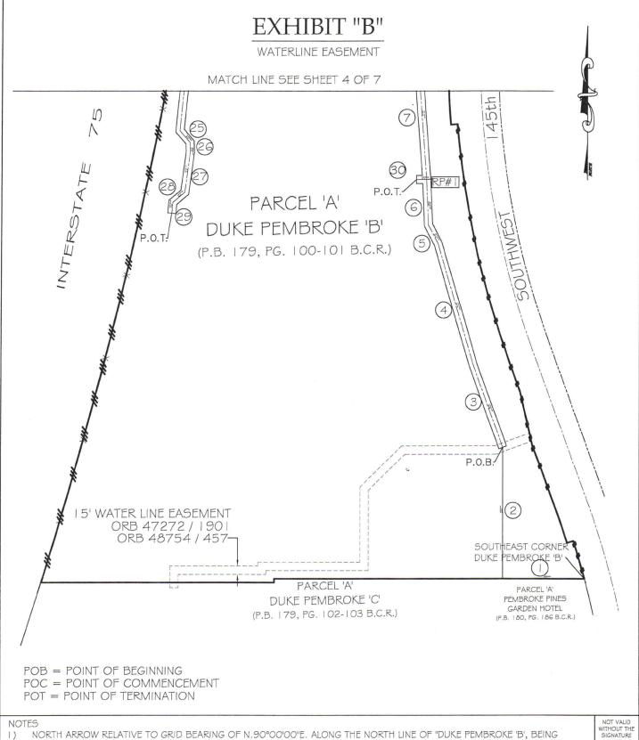
1) NORTH ARROW RELATIVE TO GRID BEARING OF N.90°00'00"E. ALONG THE NORTH LINE OF "DUKE PEMBROKE 'B', BEING ALSO THE PLAT BEARING
