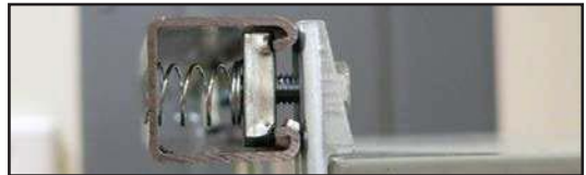
Figure 3 • Closeup of the spring nut and bolt used with the Unistrut framing bar.
