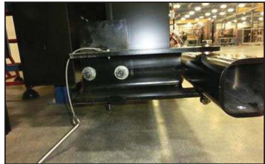
Figure 2 • Boom mounted in interface bracket and retracted to servicing position.
