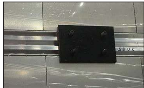
Figure 2: Bolt in bolt carrier placed into track.
