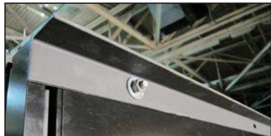
Figure 2 • Angle attached to slim cabinet mounting bolt.
