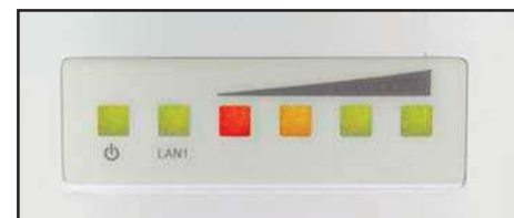
Figure 3 • LED's on the back of the radio indicate signal strength.
