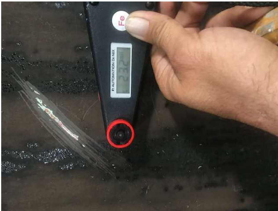
Picture 2: Adhesion and coating thickness.
