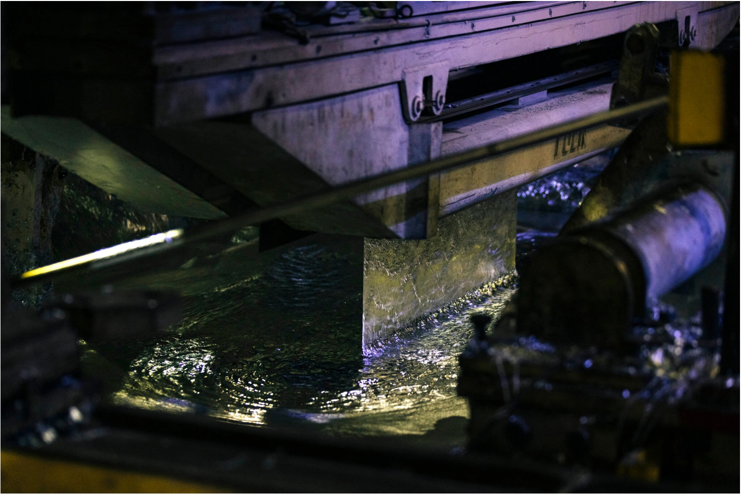
Sheets of steel are coated in zinc in the hot dip line at a Cleveland-Cliffs steel mill. Taylor Glascock for The New York Times
