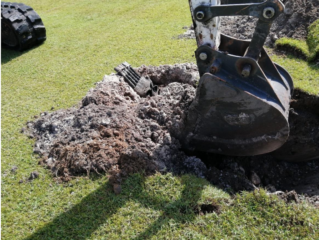
Test Pit #2: Exposed surficial soil and yard drain pipes (0-2.5 ft)
