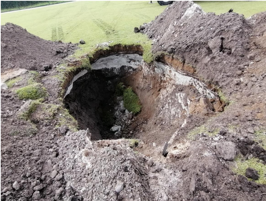
Test Pit #2: View of excavation, facing south (Note: caving occurred in the upper 7 ft)
