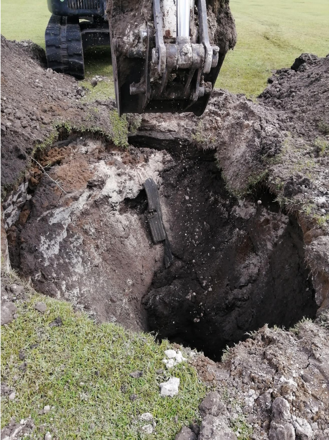
Test Pit #2: View of excavation, facing north (Note: groundwater not observed to 10+ ft and caving occurred in the upper 7 ft during excavation)
