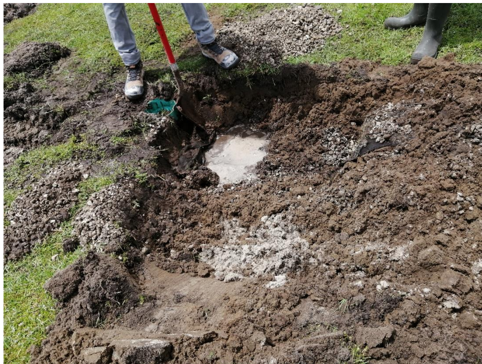
Test Pit #3: Encountered shallow groundwater on north side of the vertical drain pipe
